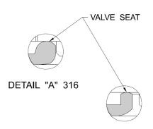
DETAIL "A" 317 (20) 2 (21) (2) 4 10 10 11 FIG. 1 19 11 13) 13 6 **6** 17 17 7 18 16 16 (8) MODEL AL316P MODEL AL317P
